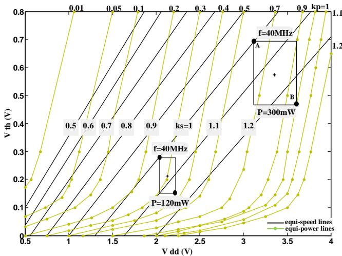
Fig. 2. Equi-power and equi-speed lines in  $V_{DD}$ - $V_{TH}$  design space
