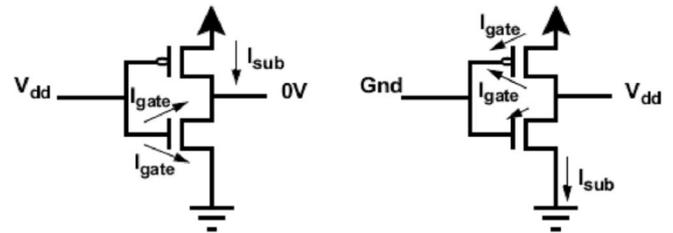
Fig. 3. Gate oxide leakage in CMOS inverter
