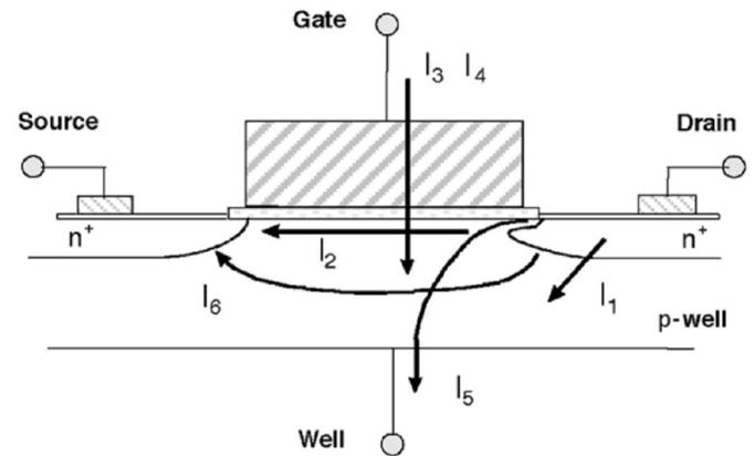
Fig. 1. Leakage current components
